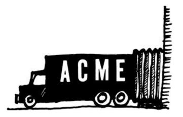
The idea of the gadget was to allow people in a building to load or unload trucks without losing cold air in the summertime or hot air in the wintertime to the out-of-doors.
